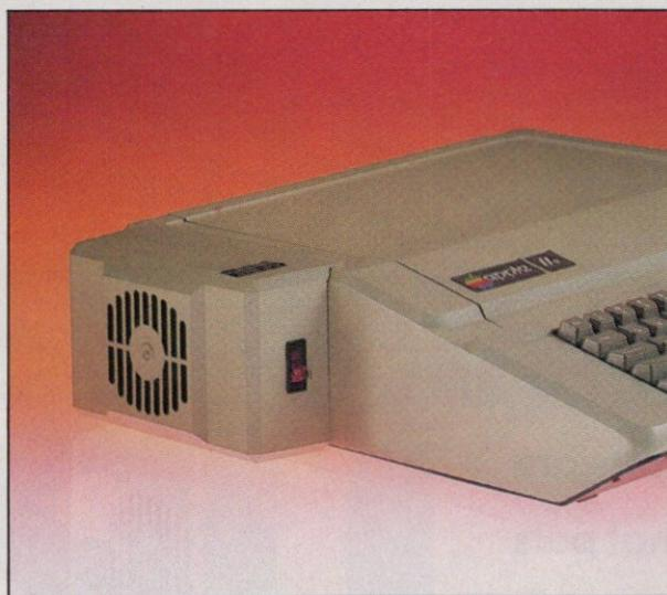
System Saver's quiet fan draws a breath of fresh air across the Apple's mother board, over the power supply and out the side ventilation slots at the rate of 17 cubic feet per minute.
